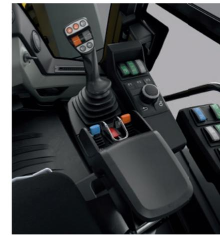
**Easily adjust hydraulic oil levels using the jog dial:**
